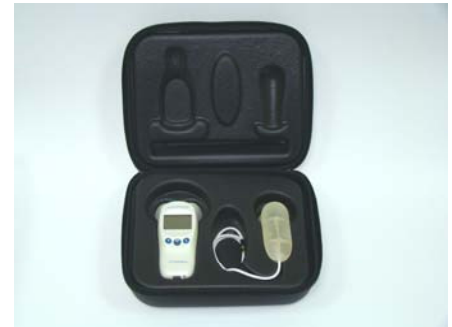
Open case showing WheezoMeter and Infant Auxiliary Sensor
